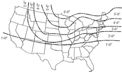
FOOTING DEPTH BELOW GRADE DIMENSION 'D'
